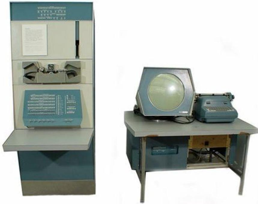
**Pictured Left to Right:** The PDP-1 Computer bays, with console display, paper tape reader and punch; and the Type 30 graphics display alongside the console typewriter. (Source: Digital Equipment Corporation) **Below:** Product Development pioneer Software Wizard Peter Samson at the console, loading paper tape. (Source: Mike Cheponis)
