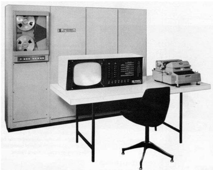
**Pictured:** *Mock-up of proposed PDP-1 product* In this case, various pieces were physically brought together to help the systems engineers appreciate some of the human factors that would need to be considered in the final design. These types of exercises are useful in getting the “what” to be better understood by all team members<sup>1</sup>. (Source: Digital Equipment Corporation, 1959)
